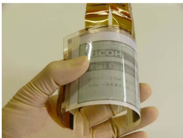
Fig. 11 Photograph of a 160 ppi flexible EPD.
