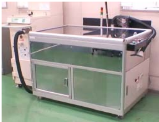
Fig. 10 Exterior view of pallet cleaner.
