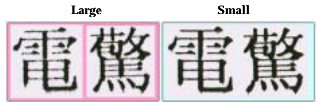
Fig.11 Comparison of character image quality on paper between different toner particle sizes
