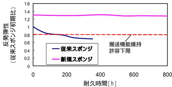
Fig.12 Transition of rebound resilience of the fusing roller by an endurance test; comparison between the conventional sponge and the improved sponge
