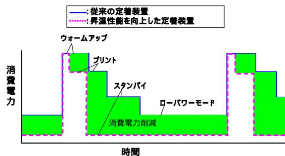
Fig.2 Transition of electricity consumption according to a regular operating mode; comparison between a conventional MFP and a target
