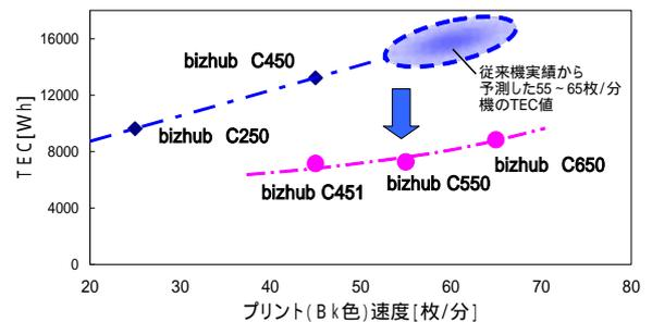
Fig.14 Comparison of TEC (Typical Electricity Consumption) value between estimation value by conventional series and result of bizhub C650/C550/C451
