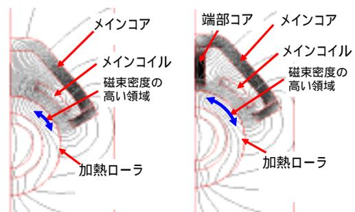
(a) Without a side core (b) With a side core
