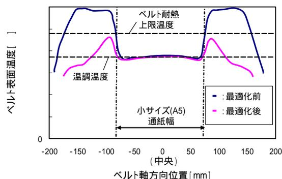
Fig.10 Experimental result of temperature distribution in the axial direction of the belt by multiple print test of narrow-sized paper;
