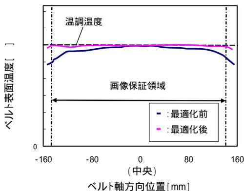
Fig. 7 Experimental result of temperature distribution in the axial direction of the belt
