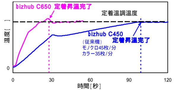
Fig.13 Comparison of rising curve of heating roller temperature between bizhub C450 and C650
