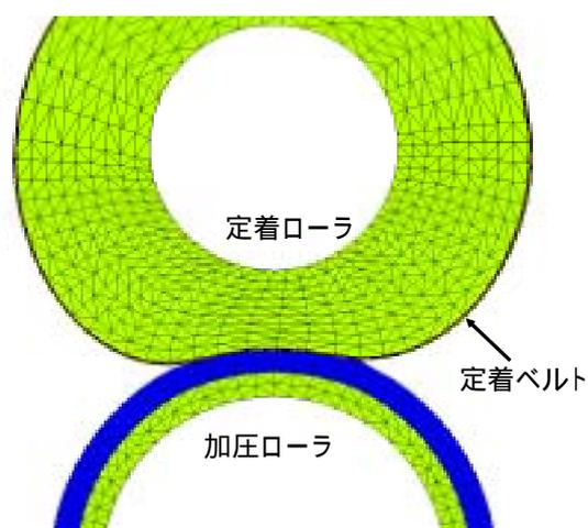
Fig.11 Fusing nip formation; simulation by the CAE analysis
